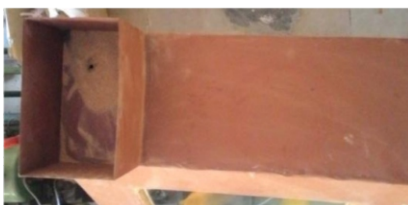
Fig3.4: Ceiling with abrasive reservoir compartment
