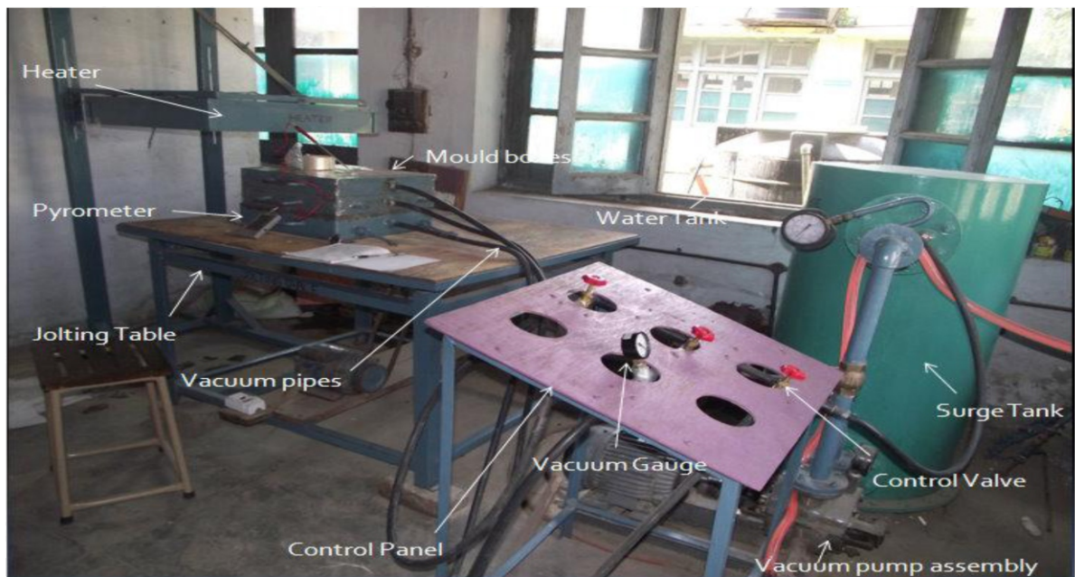
Fig. 3 3D view of VM setup
